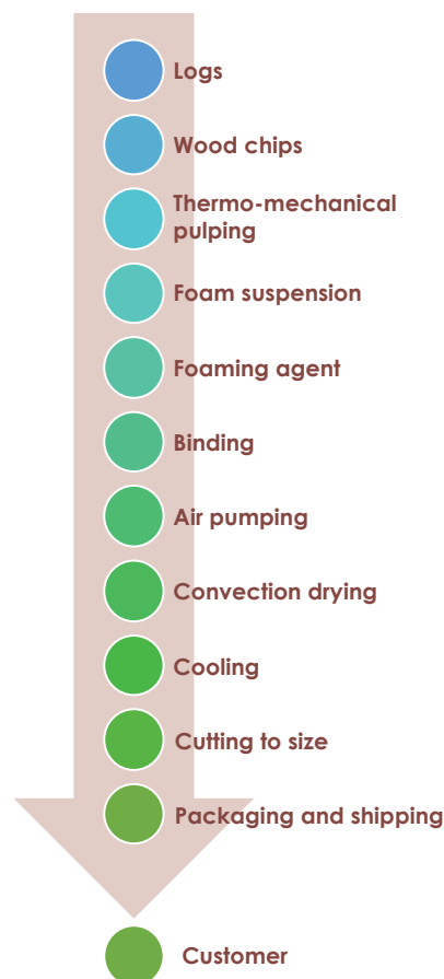
Figure 4.6. Wood foam board production process
