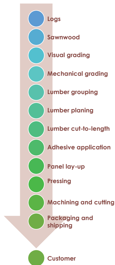
Figure 4.2. CLT production process
