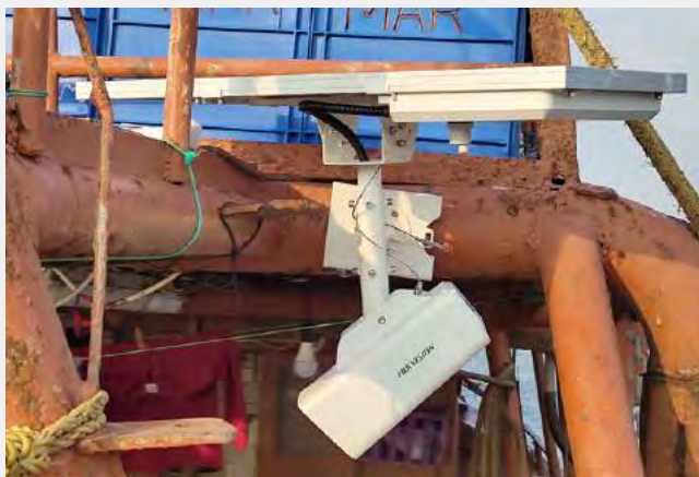
Camera with solar panel on board a fishing vessel in the Red Sea © FAO/Pedro Guemes
