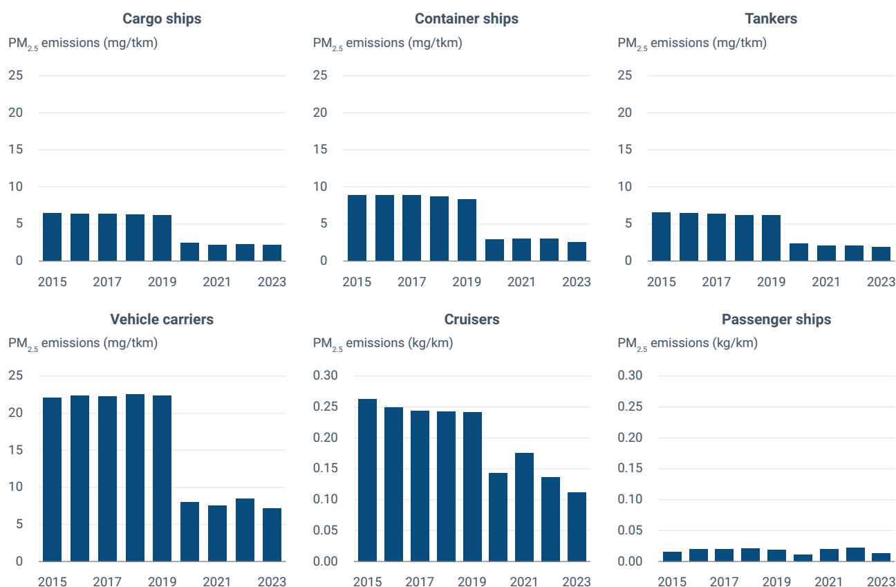
Figure 2.15 PM 2.5 specific emissions from selected freight and passenger ship types in the EU-27
